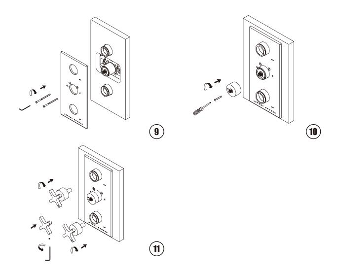
Install handle assembly with set screws.
