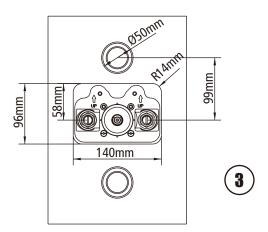
REMOVE CAP ONLY, KEEP THE REST OF THE MUD GUARD AS IT IS NEEDED TO HOLD THE TRIM FIXING SCREWS.
